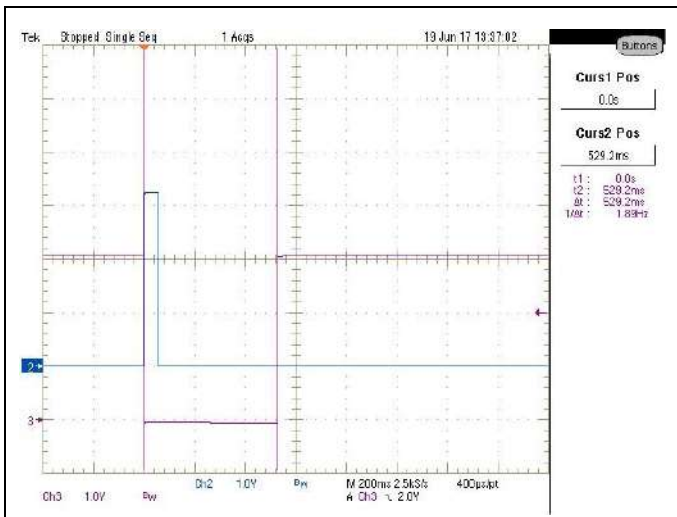
90Vac/47Hz-Min Load-Tpwok_low, CH2:,PSN, CH3:PWOK
