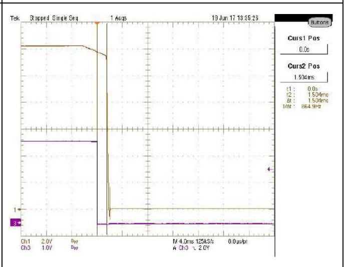
264Vac/63Hz-Max Load-Tpwok_off, CH1:12V, CH2:PWOK
