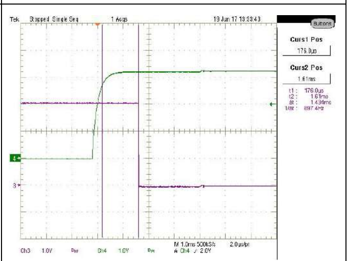
264Vac/63Hz-Max Load-Tpson_pwok, CH3:PWOK, CH4:PSON
