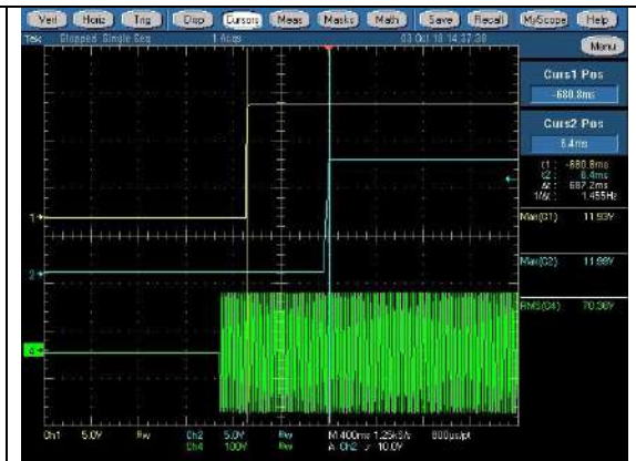
90V +12Vsb_+12V min CH1:+12Vsb, CH2:+12V, CH4:Vin
