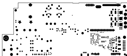
F5E062-0008 PCB P03JD5-0003IA R7 Top Solder Mask 2015/8/4
